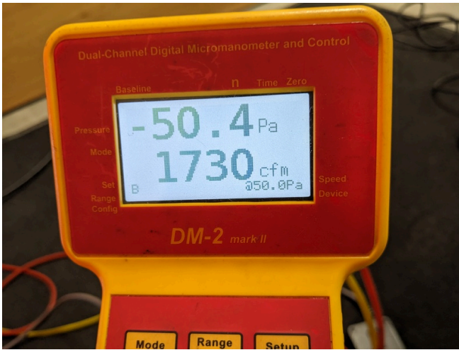
Blower Door Final Result: 1,730 CFM at -50 PA for the Whole Building
